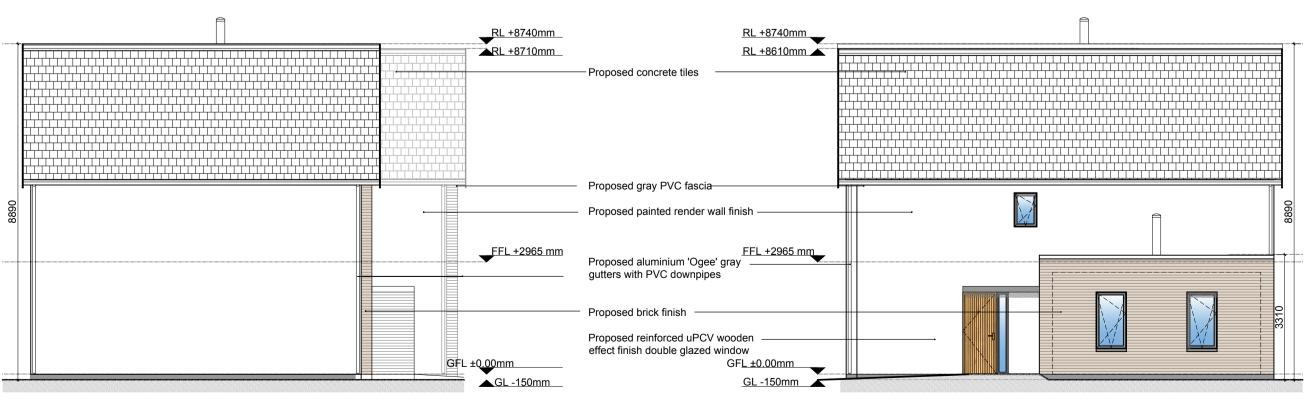
UNIT 3B PROPOSED SIDE ELEVATION Scale 1:100
